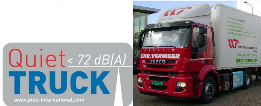
Figure 3 – The 72 dB Quiet Truck label and the first heavy truck applying for this label: a tractor running on CNG (compressed natural gas)
